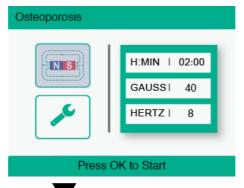
a) Press the button vso that the spanner is highlighted. At this point press OK: the display shows a moving spanner icon on the left-hand side:
