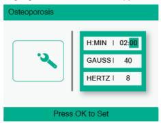
c) Use the and buttons to set the desired therapy minutes (from 0 to 59) and confirm by pressing the OK button. The display will highlight the intensity of the treatment;
