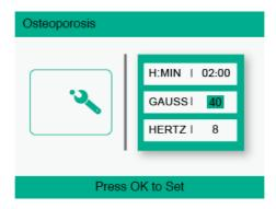
c) Use the and buttons to set the treatment intensity and confirm by pressing the OK button.
